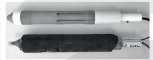
Figure 18. Photograph of angle ANZI strain cell and an overcore of the instrument installed in coal. Mills et al (2015)
